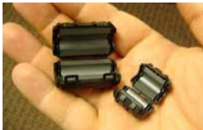
Figure 1: Your PQube meets all IEC requirements for high-frequency emissions and susceptibility, both conducted and radiated. For further protection, you can use clamp-on ferrites on signal cables to minimize radio-frequency emissions. For example, these are Panasonic KRCBC160928B and KRCBC130714B.
