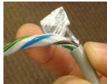
Figure 2: To minimize emissions with the optional PS1 Power Supply module, optionally use a shielded power conductor.
