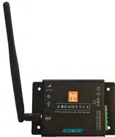
Standalone transceivers that can connect any device via RS485 and gateway
