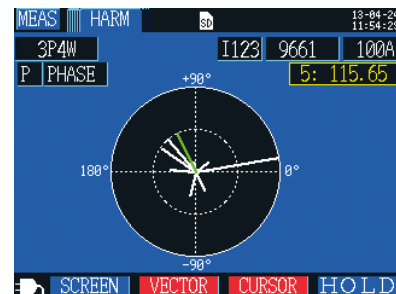
Harmonic power phase angle graph screen
