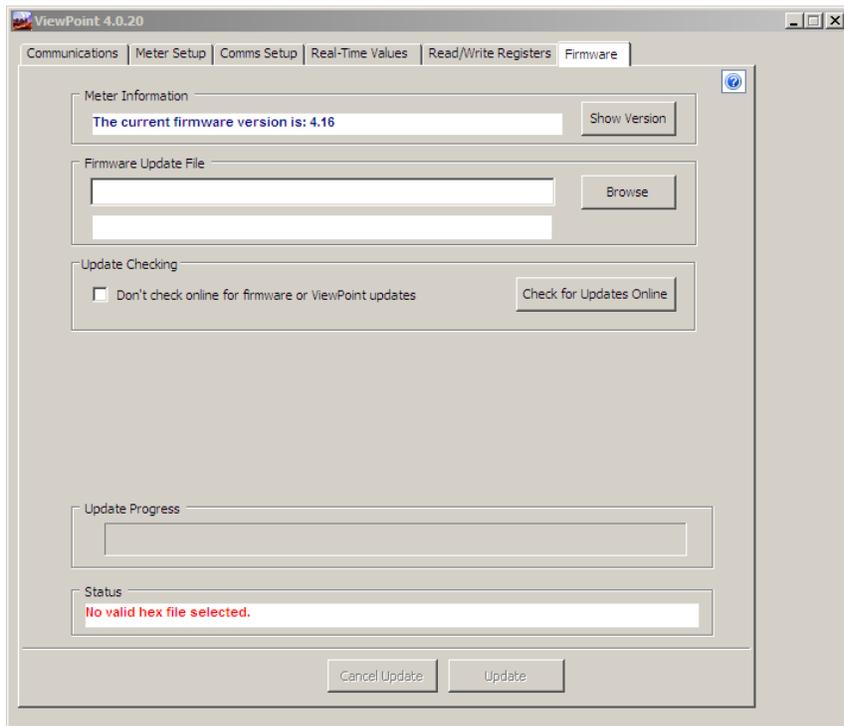
The **Firmware** screen verifies the current firmware version and updates the PowerScout internal firmware. Updating firmware is only supported in Modbus mode and is used to bring the software up to date. See the appendix *Firmware*.
