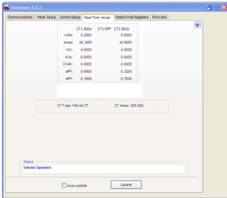
The **Real-Time Values** screen shows current readings to verify the system is configured properly. The tables display the real-time values of Volts, Amps, KW, KVA, KVAR, apparent power factor (aPF), and displacement power factor (dPF) for Phase L1, Phase L2 and Phase L3. This screen also displays the CT Type connected to the PowerScout and the CT Value.
