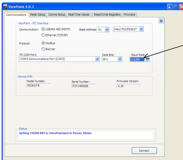
When connected via RS-485, select the baud rate of 115200.
