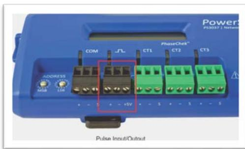
Pulse output is used to generate pulses for external devices such as data loggers that can accept pulses but do not have BACnet or Modbus capability. The PowerScout 3037 can generate pulses based on accumulated value(s) such as system kWh, system kVARh, and system kVAh. When a pulse is generated by the meter, the pulse LED will briefly flash, otherwise it will remain dark.
