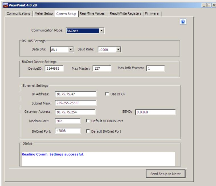
Use this tab to change communication parameters for the meter, such as communication protocols and how those communications are transferred. This screen displays the fields pertinent to your power connection and communication protocol, so if you are connected by RS-485 then only those fields are shown. However, if you are connected with a USB cable all fields are displayed. Changes to these fields override any settings on the Communications tab.
