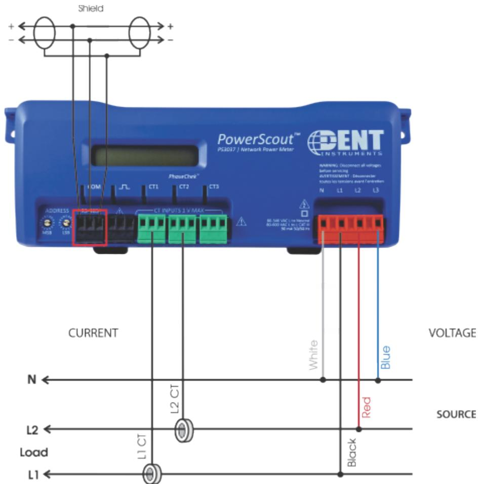
Use a Service Type **0** (zero) value for BACnet Object 12080 or a **0** (zero) value for Modbus Register 44607 on this wire configuration.
