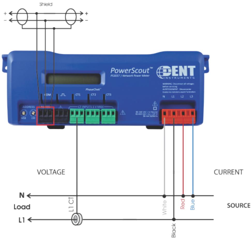
Use a Service Type **0** (zero) value for BACnet Object 12080 or a **0** (zero) value for Modbus Register 44607 on this wire configuration.
