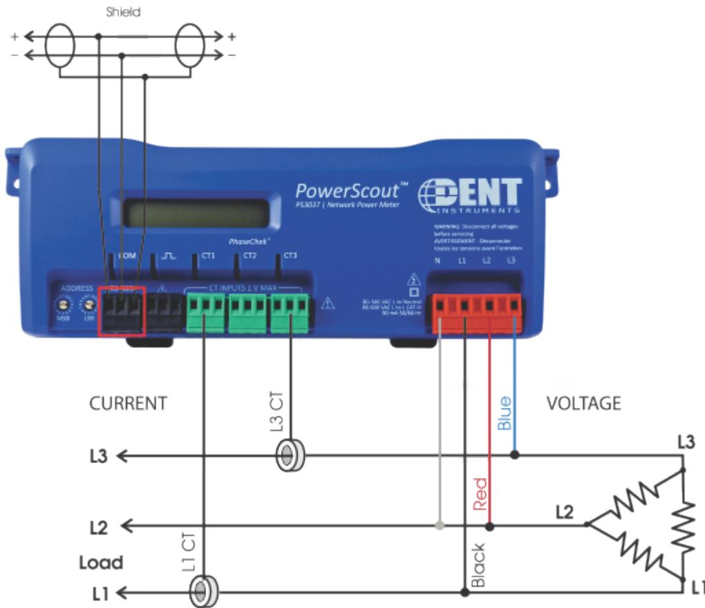
Use a Service Type **1** (one) value for BACnet Object 12080 or a **1** (one) value for Modbus Register 44607 on this wire configuration.
