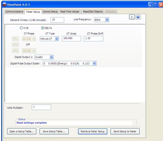
The **Meter Setup** screen allows unique changes to an element on the 3037. Within the element, *CT Phase, Type, Amps, and Phase Shift* are entered, based on wiring connection, for CT1, CT2, and CT3. The type of wiring connection and the *Digital Output* are also entered for the element. Overall, a *Demand Window* of 1–60 minutes is available for the recording of values and a *Line Frequency* of 50 Hz or 60 Hz is selectable.
