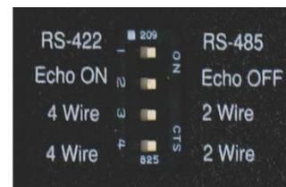
Figure II-2: Dip switches on back of RS-485 Adapter
