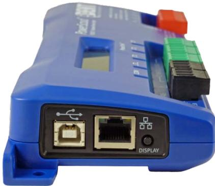
Keep in mind that the Ethernet connection must have an IP Address in the ViewPoint software that can either be set manually within the software with the *Use Static IP* address option (for a fixed address) or obtained automatically from the router connected to the logger using the *Use DHCP* option (dynamic address). Both options have advantages. See **About IP Addresses** further in this document.
