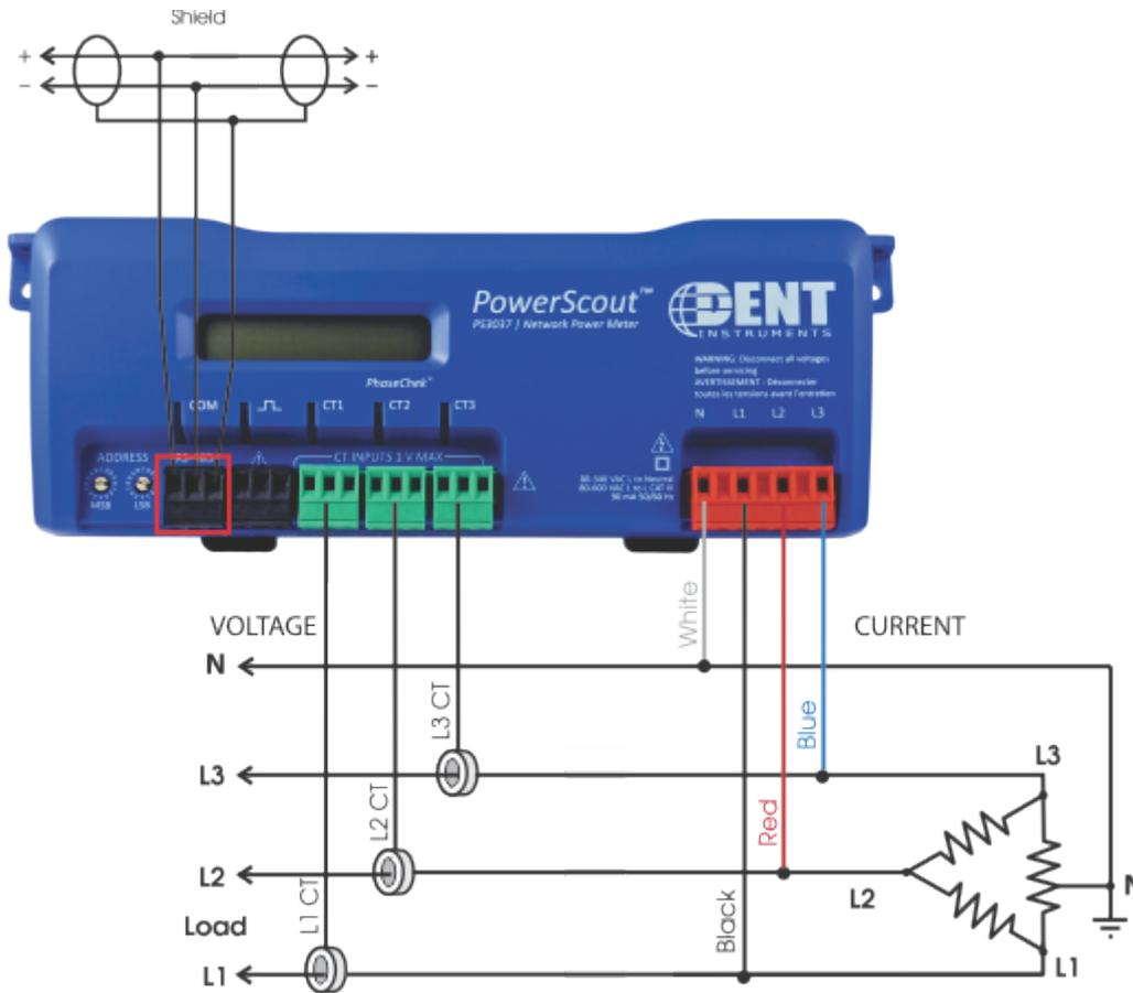
Use a Service Type **0** (zero) value for BACnet Object 12080 or a **0** (zero) value for Modbus Register 44607 on this wire configuration.
