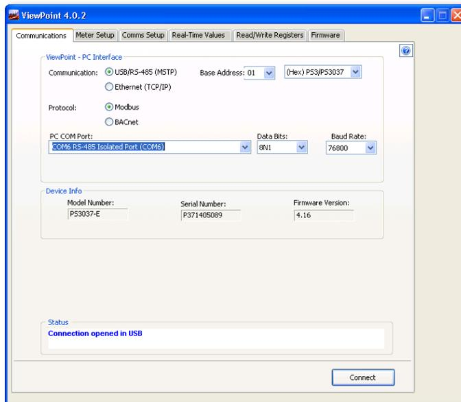
ViewPoint can read information through a USB, an RS-485 isolated COM port, or an Ethernet connection. When the RS-485 connection is selected a base address is required (the base address is the rotary switch settings). Address switches are ignored by both USB and Ethernet. When the Ethernet connection is selected an IP address is required. The screen display changes based on your connection selection.
