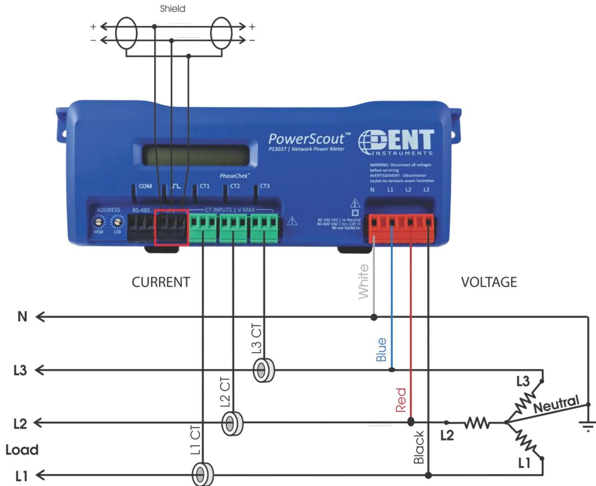
Use a Service Type **0** (zero) value for BACnet Object 12080 or a **0** (zero) value for Modbus Register 44607 on this wire configuration.
