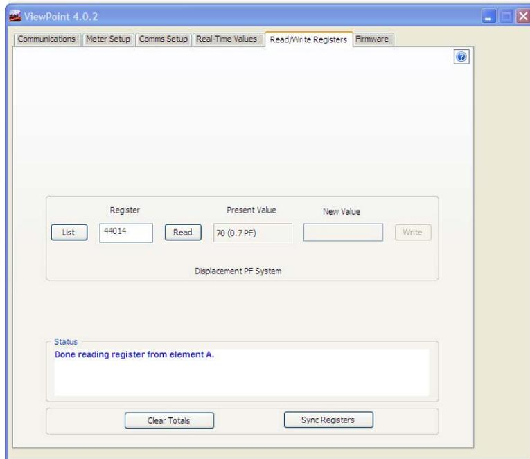
The **Read/Write Registers, Read/Set Objects** screen provides diagnostic and special configuration options, allowing the changing or viewing of the value of any PowerScout register or object. The tab name changes depending on what protocol (Modbus or BACnet) you are using. Its use is not required for a basic setup.
