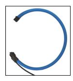
Place the flexible coil around the cable or buss bar to be measured and close the coil by clipping together the contacts.
