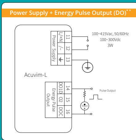
Note: \*\* Wiring diagram is only applicable to Acuvim BL.
