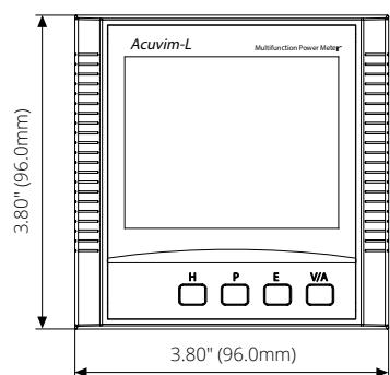
Front View of the Display Meter and Remote Display Unit
