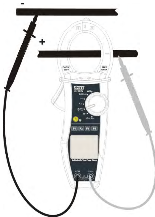
Fig. 11: DC power measurement
