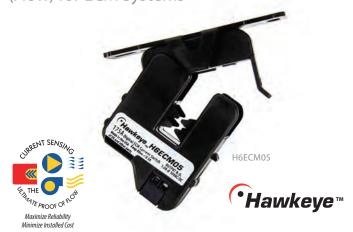
The H6ECM is a current-sensitive switching device that monitors current (amperage) in the conductor passing through it. A change in amperage in the monitored conductor that crosses the switch (setpoint) causes the resistance of the FET status output to change state, similar to the action
