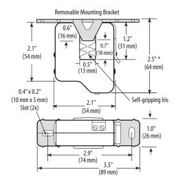
$<sup>^{*}</sup>$  Terminal block may extend up to 1/8" over the height dimensions shown.
