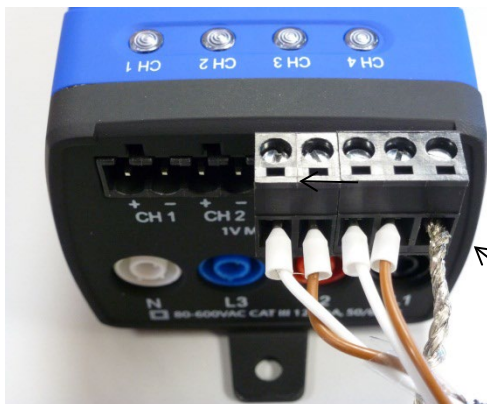
Connecting RōCoil CTs to an ELITEpro XC
