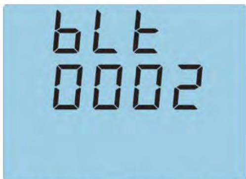
Fig 3.27 LCD back light time setting
