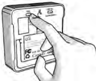
Wireless energy monitor link button
