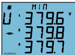
Fig.3-25 Min value of phase voltage
