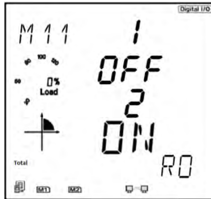
Figure 5-29 Relay Output Status Readings
