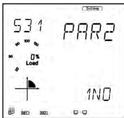
Figure 5-54 Parity setting for the AXM-RS485 module
