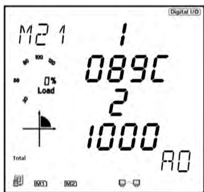
Figure 5-37 Analog Output readings from the meter's display
