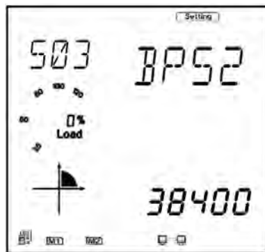
Figure 5-53 Baud Rate setting for the AXM-RS485 module
