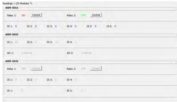
Figure 5-32 Relay Output Readings from Acuvim Software
