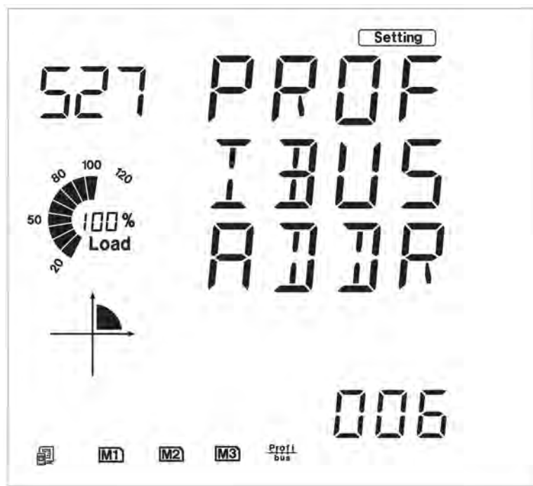
Fig 5-55 Address setting of PROFIBUS module
