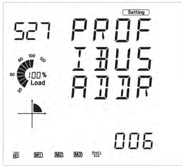
Fig 5-55 Address setting of PROFIBUS module
