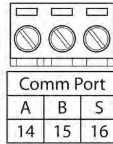
Fig 2-5 Terminal Strips of Acuvim II series meter
