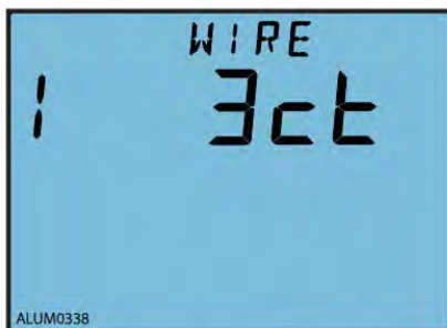
Fig.3-41 Current input wiring setting
