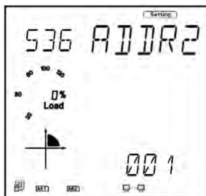
Figure 5-55 Address setting for AXM-RS485
