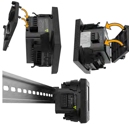
Figure 2-13 – Install the AXM-DIN rail adapter
