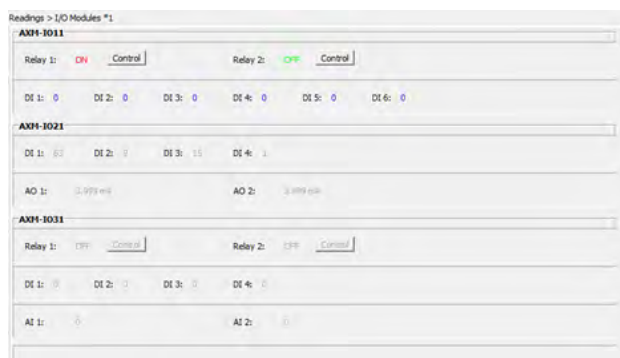
Figure 5-32 Relay Output Readings from Acuvim Software
