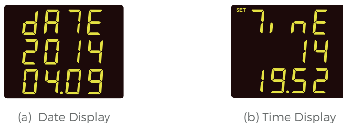
Fig 4-6 Clock Information Display
