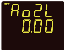
Fig 3-23 AO2 Lower Limit Setting
