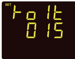
Fig 3-30 RO1 Alarm Delay Setting
