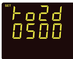
Fig 3-32 RO2 Momentary Delay Time
