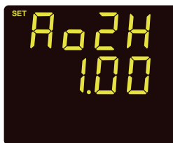
Fig 3-24 AO2 Up Limit Setting
