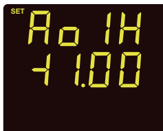
Fig 3-21 AO1 Up Limit Setting
