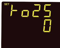
Fig 3-34 RO2 Alarm Inequality Setting
