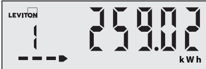
Figure 7 - LCD Appearance in Proper Operation (Example)
