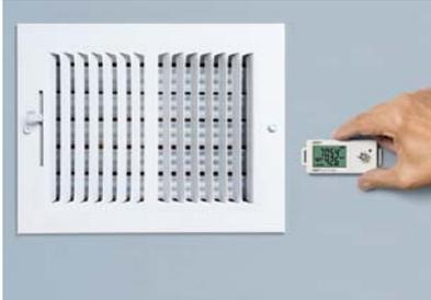
Stand-alone data loggers are compact and easy to set up and deploy. You have a choice of low-cost, stand-alone loggers with internal sensors for measurements at the logger location, or multi-channel loggers with external sensors for monitoring at some distance from the logger. All standalone loggers communicate with a PC or Mac via USB.
