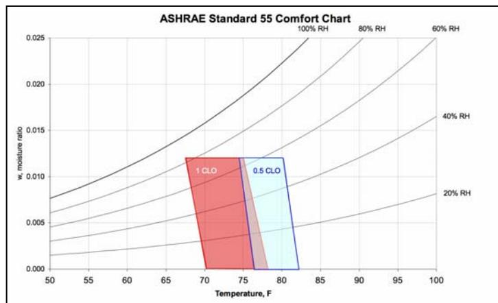
When evaluating a space for comfort, use a data logger that records air temperature and relative humidity in 15-minute intervals and compare the results to the Standard 55 comfort chart. When placing data loggers, consider the following factors:
