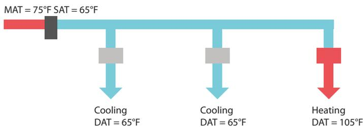
Historically, cooling systems without supply air temperature reset are designed and configured to deliver 55°F air without considering whether this temperature provides optimum performance or comfort. Further, building operators often respond to hot complaints by reducing supply air temperature (where possible) to satisfy one or two zones, but fail to realize the detrimental effect this may have on the balance of the system and occupants.
